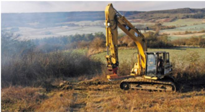
Mechanical shrub-clearing using an excavator
